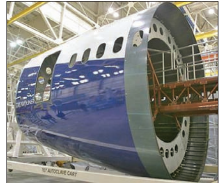
Figure 1. Carbon fiber composite barrel used on Boeing 787.
